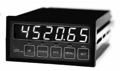
**Orbit Controls Model OC7166** is a 6 digit dual counter with two inputs P and S. The two counters operate independently from each other. The common display can be selected to show the results of the counter P or the counter S, the addition P+S, the subtraction P-S, the multiplication PxS or the division P:S. The display function is selected with the keypad at the front.
